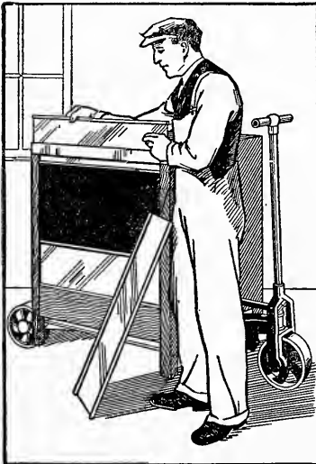
ADJUSTING A BIN TO THE LOAD Rough parts and small castings carried in bulk are easily accessible in this steel skid-box with adjustable sides
